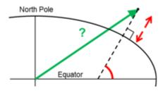
Geodetic latitude, longitude and height are given for position B as latEB, lonEB and hEB, find the ECEF-vector for this position, p\_EB\_E.
