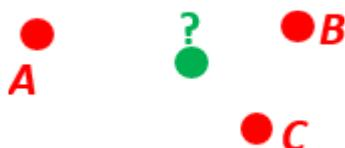
Three positions A, B, and C are given as n-vectors  $n_{EA\_E}$ ,  $n_{EB\_E}$ , and  $n_{EC\_E}$ . Find the mean position, M, given as  $n_{EM\_E}$ . Note that the calculation is independent of the depths of the positions.
